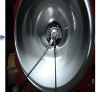
Reflector with Xe-Arc Lamp
