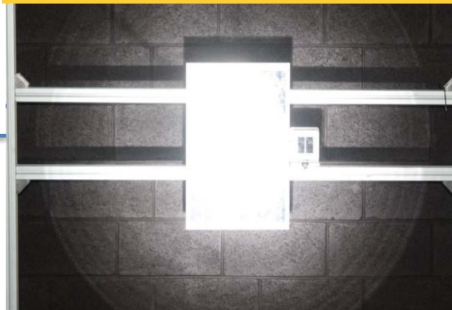
Target Area with Reference cell and C-Si Module
